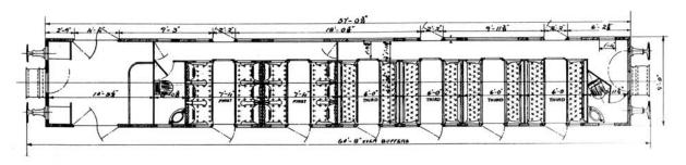
Weight 30t 0c, seating  $12(1^{st})/32(3^{rd})$  in 2/4 compartments. Built by R.Y. Pickering, Wishaw, with simple paneling and angle truss underframes.
