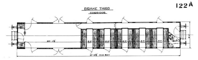
Weight 30t 0c, seating 40 in 5 compartments. Built by R.Y. Pickering, Wishaw, with simple paneling and angle truss underframes.
