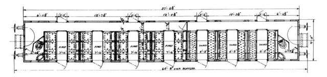
Weight  $30t\,0c$ , seating  $24(1^{st})/24(3^{rd})$  in 4/3 compartments. Built by R.Y. Pickering, Wishaw, with simple paneling and angle truss underframes.
