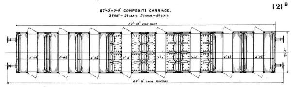
Weight 28t 17c, seating  $24(1^{st})/60(3^{rd})$  in 3/5 compartments. Numbers 452-459 built by Clayton Wagons Ltd., Lincoln, the remainder at St. Rollox all with simple paneling and angle truss underframes.
