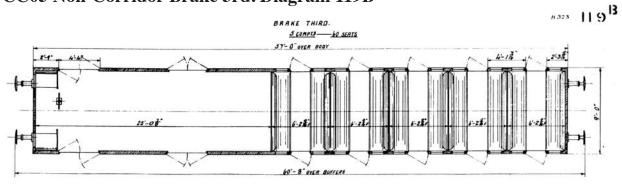
Weight 27t 10c, seating 24 60 in 5 compartments. Specifically for Lots H349-357 [earlier lots had a different style of underframe while later lots had simple paneling!] built at St. Rollox with full paneling and round bar and queenpost underframes.
