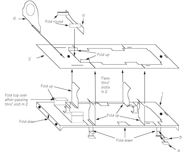
9.7 Bend the steps as shown in the diagram below and fit the treads (parts # 3 and 4) after folding each into an L shape. Reinforce the rear of the sub-footplate/step joint with a fillet of solder. The prototype had a brace rod as shown which may be simulated with a length of wire.
