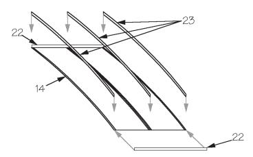
11.25 Curve the roof (part #154) to match the profile of the cab front. Fit the stanchions (parts #23) and the roof side strips (parts #22) as shown in the diagram. The roof is probably best not fitted in place until the final assembly.
